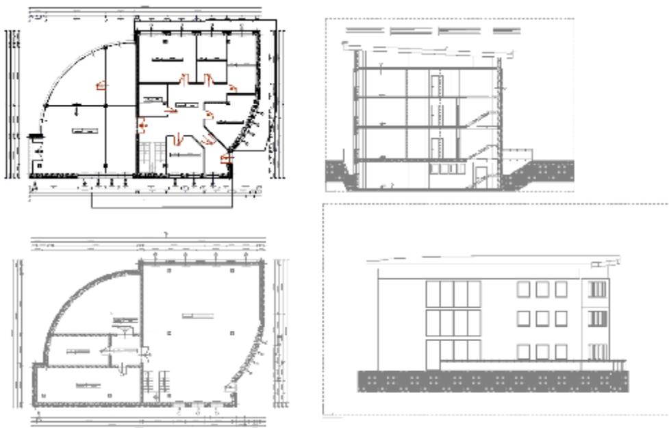
Drawing 11. Views with only one level enabled in each view.
